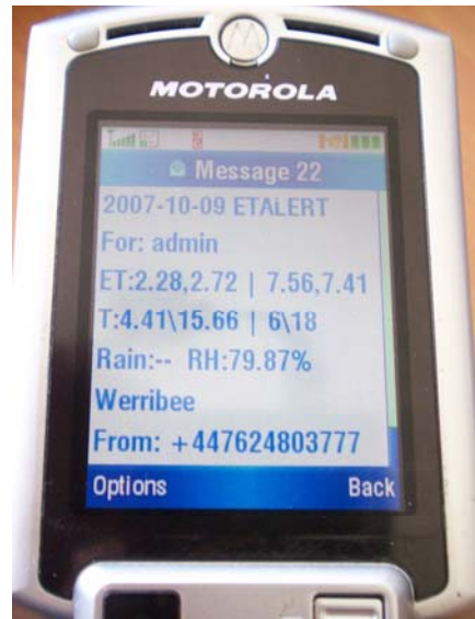
Through SMS to view ET rate, min. and max. Temperature, rainfall and relative humidity
